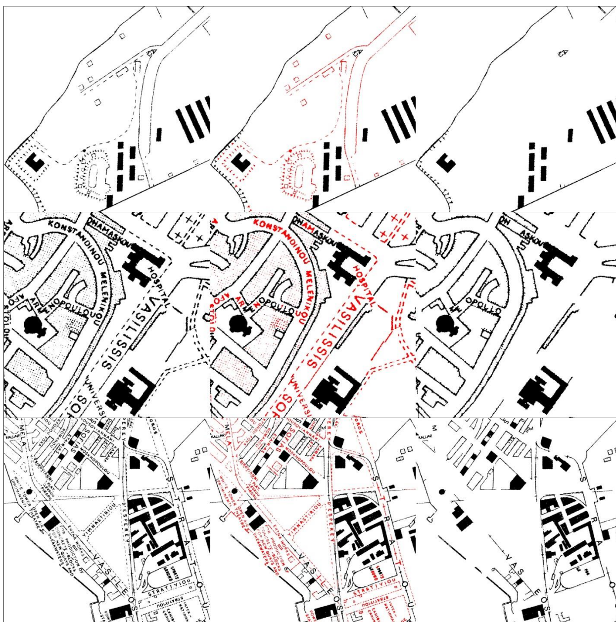
Figure 5. Left – binary image, Center – clumps marked as red, Right – binary cleaned image
