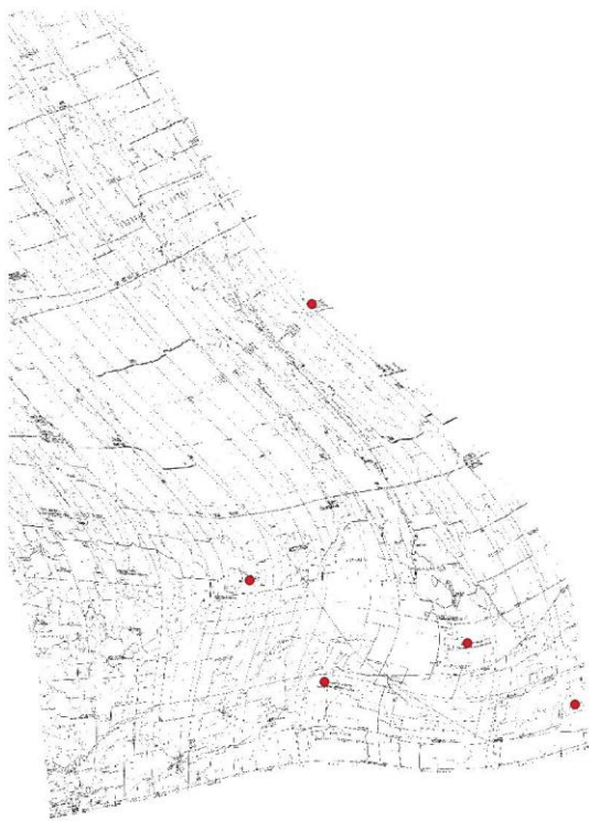
Figure 4. Misplaced GCPs because of geocoding equating township names and settlement names. Map: USGS Aitkin (1994).
