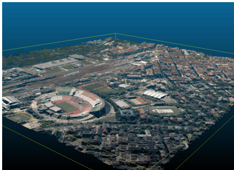
Fig. 28 Digital surface model (DSM), Colorized point-cloud
