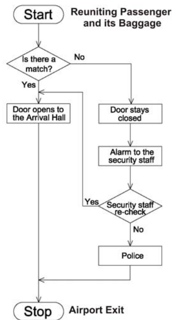
Figure 27: Simplified Flowchart Diagram for Passenger and Baggage Identification Machine at the Baggage Claim (Source: Own Research)
